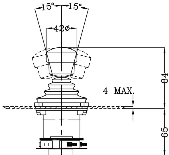
THE V10 BANG BANG MASTER SWITCH IS DESIGNED FOR RADIO AND PORTABLE CONTROLS. IT IS SMALL, LIGHTWEIGHT AND SOLID IN DESIGN. IT IS BUILT FOR 6 MILLION OPERATIONS. IT IS OIL, OZONE, UV AND SALT ATMOSPHERE (OCEAN CONDITION) RESISTANT. CONTACTS ARE RATED AT 16A 250VAC DEGREE OF PROTECTION FRONT: IP54
