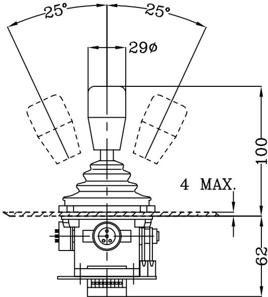
THE V10 MASTER SWITCH IS DESIGNED FOR RADIO AND PORTABLE CONTROLS. IT IS SMALL, LIGHTWEIGHT AND SOLID IN DESIGN. IT IS BUILT FOR 6 MILLION OPERATIONS. IT IS OIL, OZONE, UV AND SALT ATMOSPHERE (OCEAN CONDITION) RESISTANT. CONTACTS ARE RATED AT 5A 30VDC DEGREE OF PROTECTION FRONT: IP54
