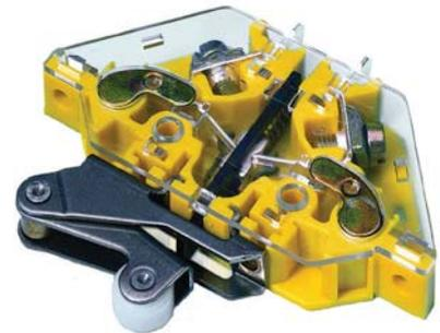
Several contact blocks can be plugged on the top of each other and operated jointly. The plug-type terminals are then only accessible on the top unit. The contact blocks can be provided with shock protection to DIN VDE 0106 Part 100.
