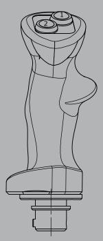
**B15**Push button installed Pos. 1,2
